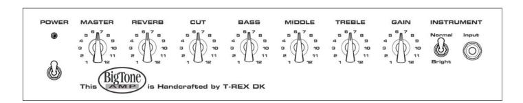
POWER SWITCH: ON/OFF (outer positions): Turns the amplifier ON/OFF.
